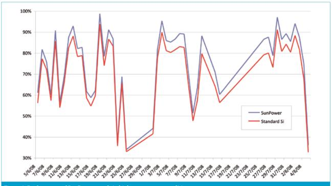
Figure 8. Performance of SunPower panels in high temperature conditions.
